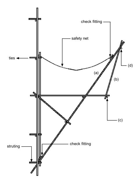
Notes: (1) The net and its supporting framework are attached to the scaffolding structure which should be securely tied back to the building.
