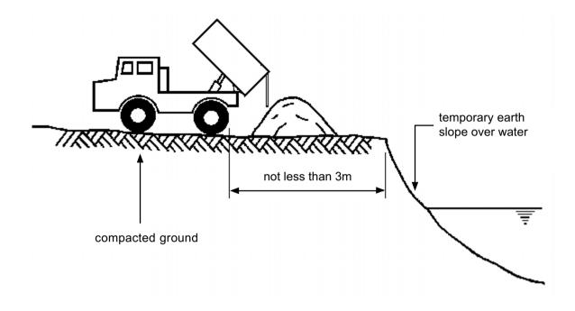
Notes: (1) Materials should be deposited on the surface of compacted ground.
