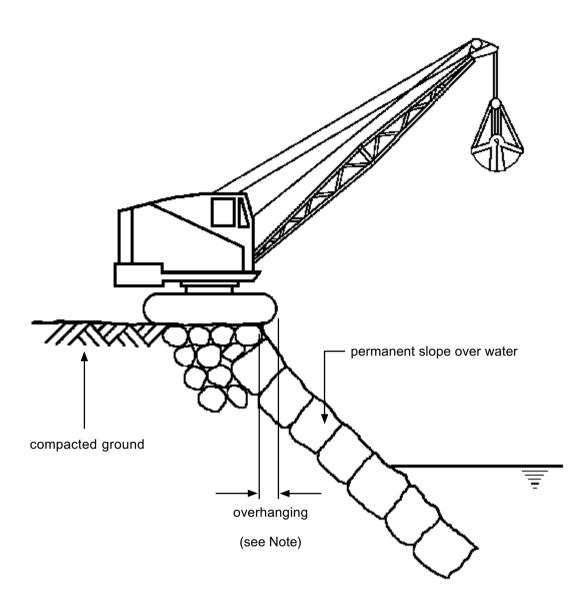
Note: Overhanging of any part of the crawler tracks or wheels should not be permitted.
