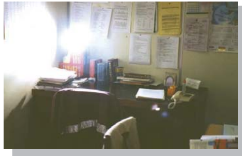
Fig. 2a Disability glare from a light fitting
