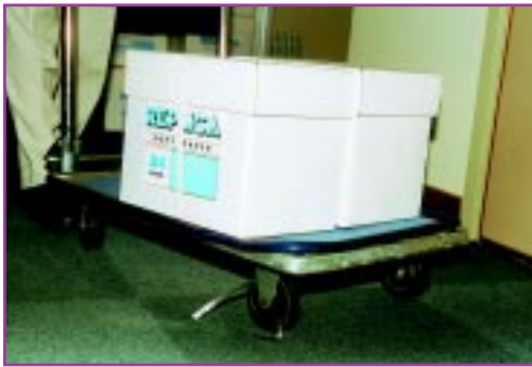
It is harder for the operator to pull or push when wheels are not properly maintained.
