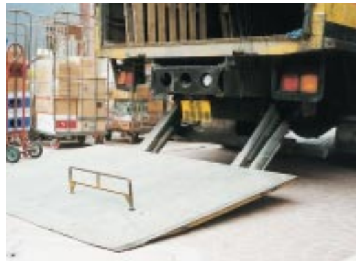
Installing a guard on the tailgate prevents trolleys from sudden movements.
