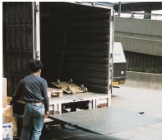
Using a truck's extended tailboard makes manual handling much easier for workers.
