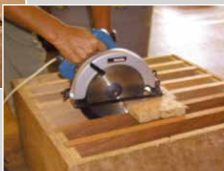
Portable electric saw with protective guard and workpiece holder for decoration works
