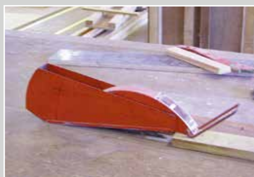
Bench circular saw fitted with adjustable top guard and riving knife
