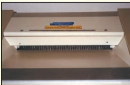
Shredders consist of revolving cutters located behind the machine casing. Without proper guarding, the operator's finger may slip through the feed opening and get hurt by the revolving cutter. Likewise loose clothing or long hair of an employee operating the machine can easily be dragged into the slot and entangled by the revolving cutter. The dangerous part should be effectively guarded as shown below.
