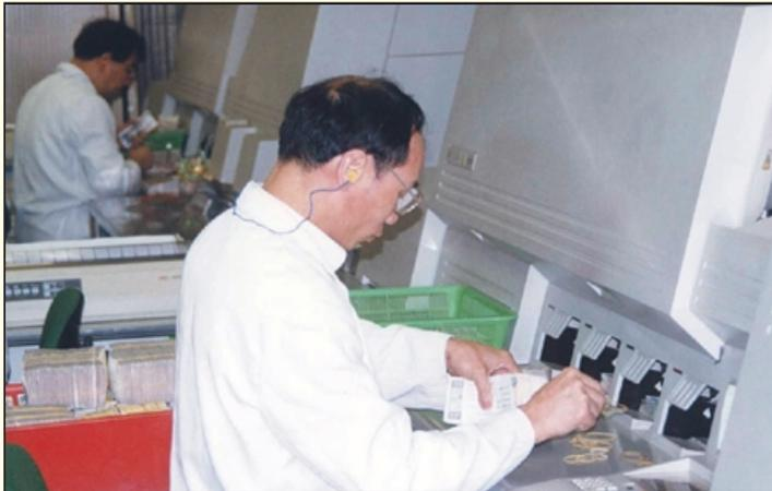
The automatic banknote counting machine can be housed inside a separate room to contain the noise emitted by the pneumatic bank-note delivery system. Hearing protectors should be worn by the workers attending to the machine.
