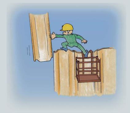
**b.** Strike by a hoisting sheet pile during the interlocking operation, in particular, in a windy condition
