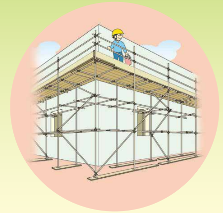
Double row scaffold and working platform
