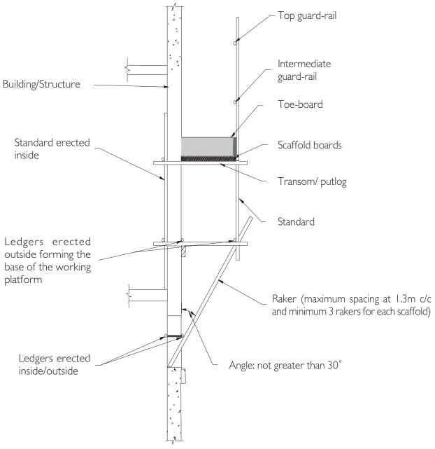
(i) For the top guard-rail: at a height between 900mm and 1,150mm above
