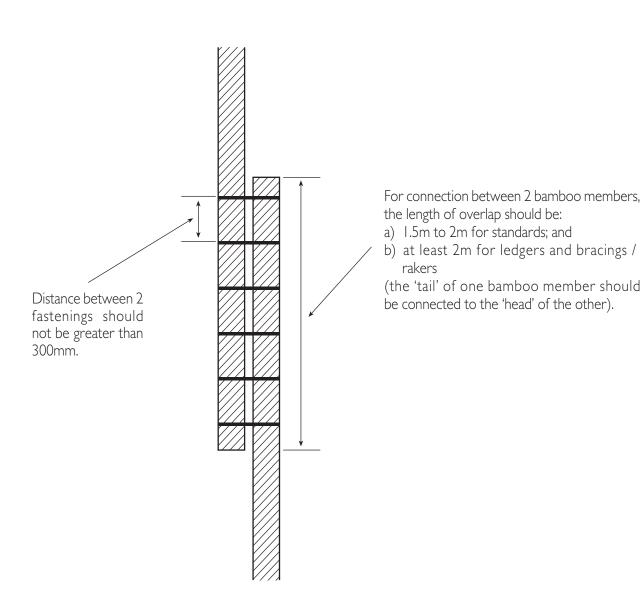
Figure 7: Single lift type truss-out bamboo scaffold (side elevation – not to scale)
