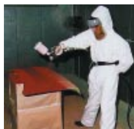
If chemicals can contaminate the whole body, full body protection is required, such as a face shield, coveralls and gloves.
