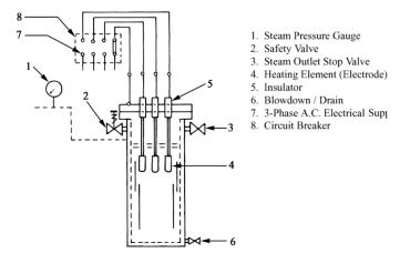
Electrode Type Electric Steam Boiler
