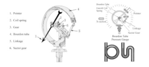
The Competent Person is required to observe the pressure shown on the pressure gauge. Therefore, the gauge must be accurate. To ensure the accuracy, the pressure gauge must be calibrated as necessary and at least at the time of periodic survey.
