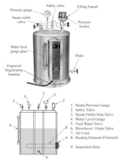
Manually Controlled Filament Type Electric Steam Boiler
