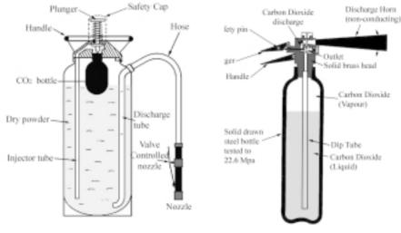
Fig.1 Dry Powder Fire Extinguisher Fig.2 CO<sub>2</sub> Fire Extinguisher
