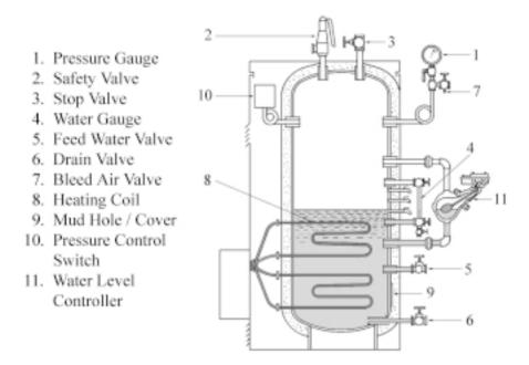
Automatically Controlled Filament Type Electric Steam Boiler
