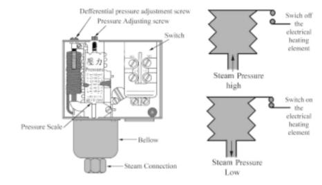
Pressure Switch for Steam Pressure Control
