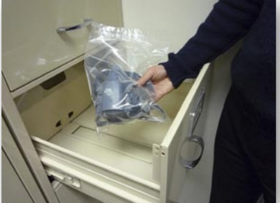
Keeping a bagged RPE in a locker to avoid disturbance or contamination
