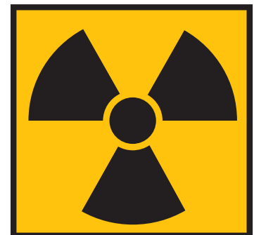
The above sign indicates presence of ionizing radiation.
