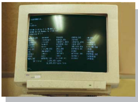
Fig. 3 Veiling reflections: the reflection of the lights is masking information on the screen.
