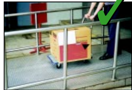
Using a ramp or adding a temporary ramp reduces the risk of accidents.
