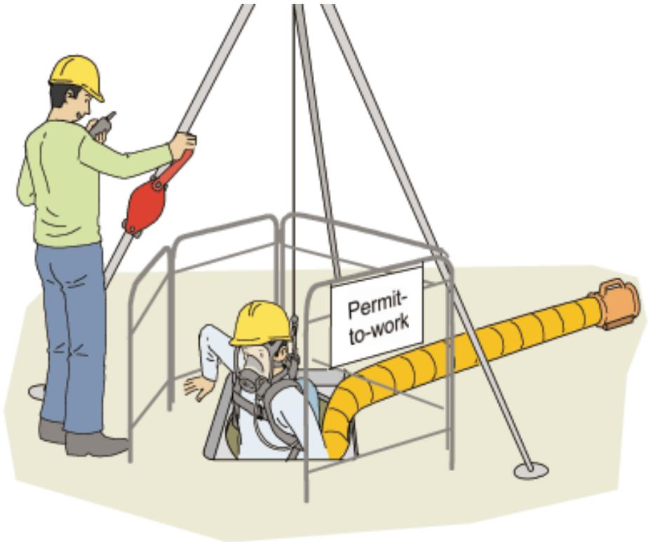
*The standby worker should station outside the manhole and maintain constant communication with the certified worker inside.*
