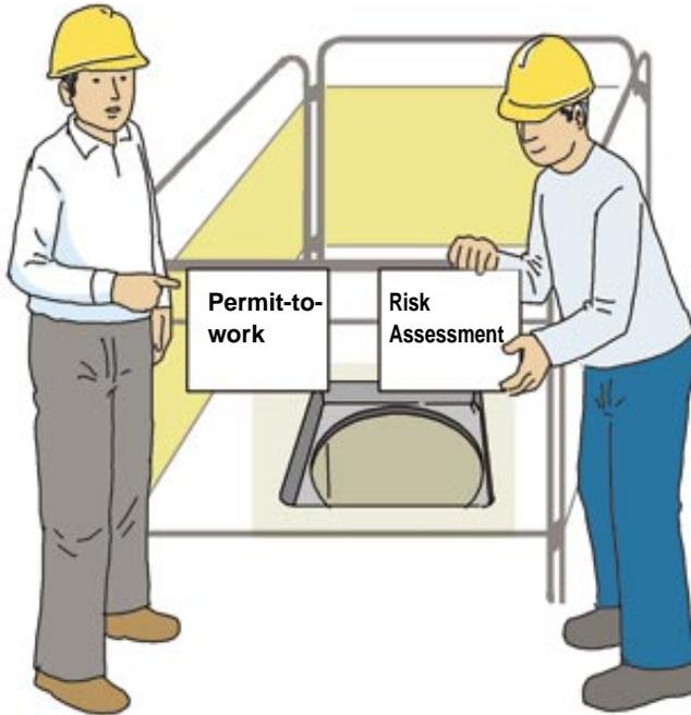
*Entry into a manhole for work should be permitted only after the issue of a valid permit-to-work certificate.*
