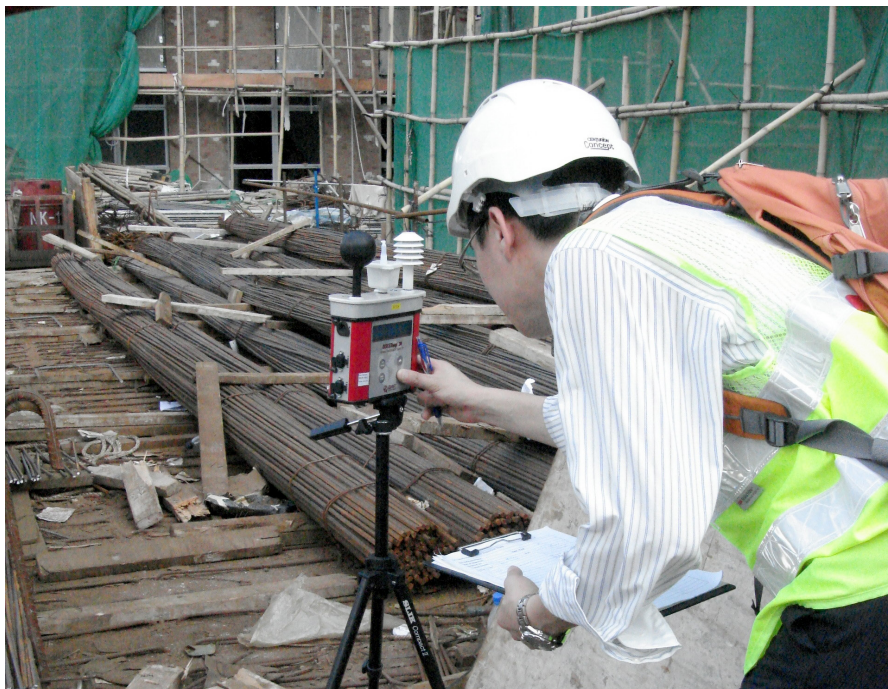
An occupational hygienist measuring the heat stress level in a construction site
