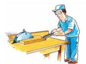
• The blade catches the timber and violently throws it back to the front of the saw, towards the operator.
