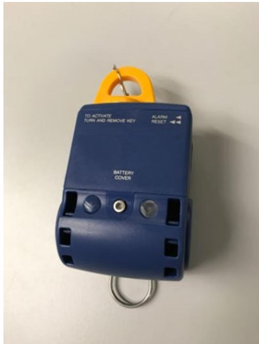
Photo 4 - Personal distress alarm (motion sensor)
