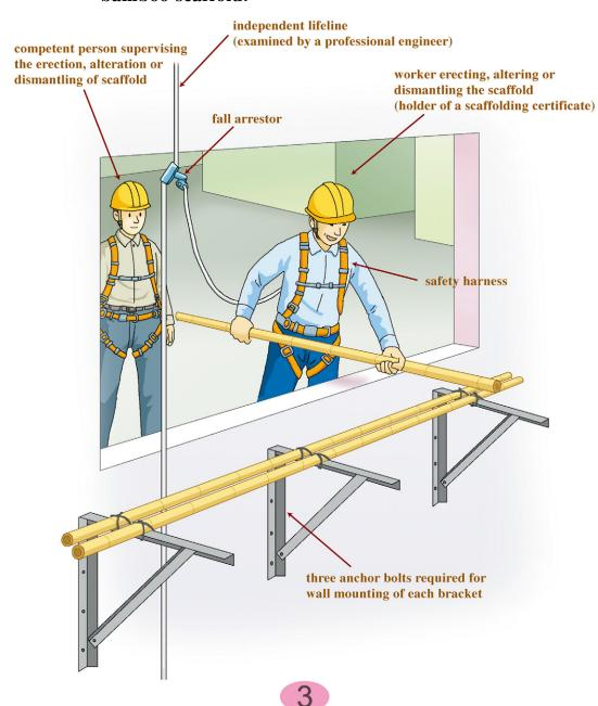
Safety harness must be attached to an independent lifeline examined to be safe by a professional engineer. It must not be secured to any window frame, window hinge or insecure anchorage point.
