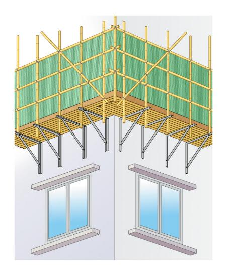
This type of scaffold must be designed by professional engineers and erected, altered or dismantled by trained workmen with adequate experience under the immediate supervision of a competent person. Report of results of scaffold inspections under the Construction Sites (Safety) Regulations 检查省簽署及程標 Signature and designation of erson who made the inspection
