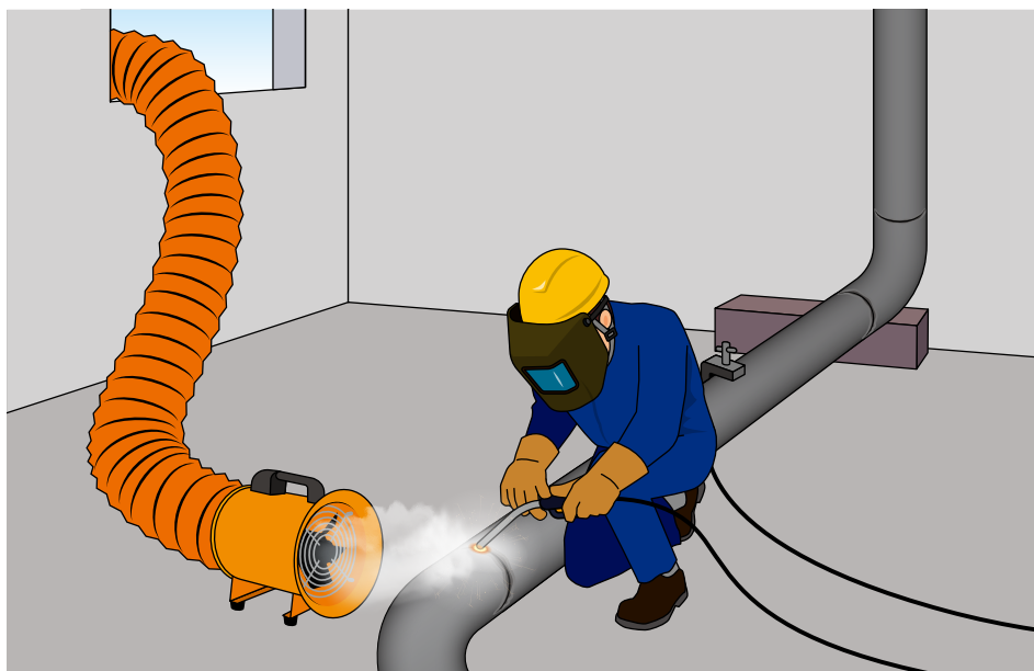
An LEV system can be used during the welding process to remove contaminants
