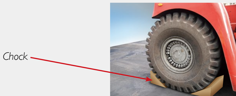
Figure 7 The wheel is fixed with chocks
