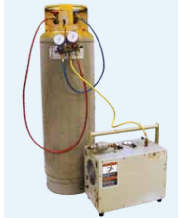
Refrigerant recovery equipment
