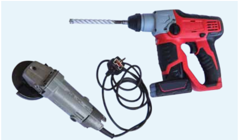
Electrical tools should function properly, insulation material or casings should be intact
