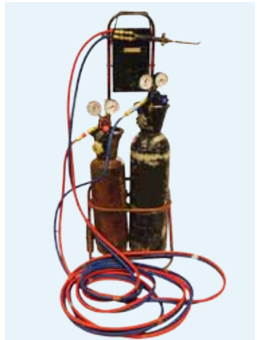
Oxy-acetylene welding set
