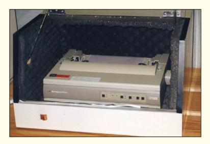
An acoustic booth can be used to isolate noisy equipment such as the above pin-writers and an old fax machine.
