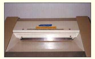
A **transparent** plastic sheet reduces the feed opening of the shredder to its minimum size.
