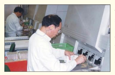
The automatic banknote counting machine can be housed inside a separate room to contain the noise emitted by the pneumatic bank-note delivery system. Hearing protectors should be worn by the workers attending to the machine.
