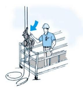
A suspended working platform should be installed with a safety rope with an automatic safety device mounted on it. No person shall tamper or interfere with or render inoperative such safety rope and automatic safety device.
