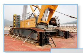
▲ Lifting appliances/mobile plant should be kept away from dangerous locations such as openings, edges close to water.
