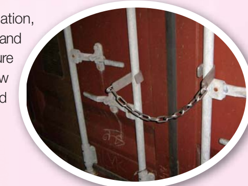
A device to secure the doors of a freight container in position
