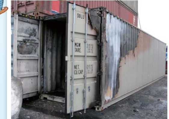
Explosion and fire caused by waste plastic materials in a freight container
