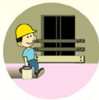
Provision of guardrails & toe-boards at lift shaft openings
