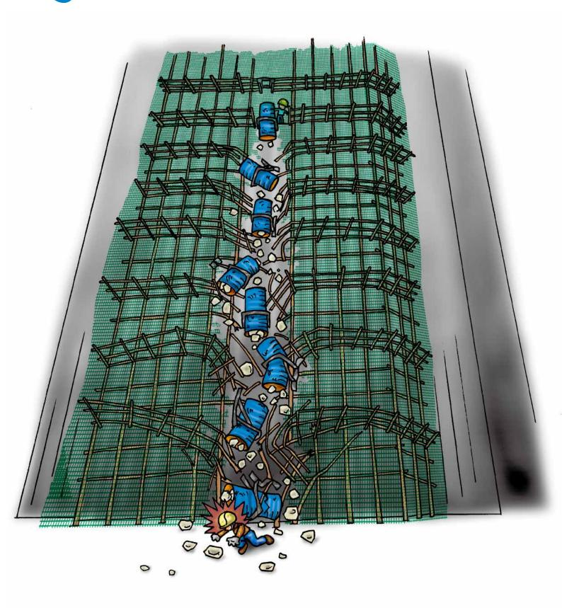
In a building renovation site, refuse chutes were installed on the external walls of the building for removal of debris from the upper floors. At the time of the accident, waste mosaic tiles were being removed from the upper floors to the ground with the use of the refuse chutes. The accident happened when one of the refuse chutes collapsed. The refuse chute and debris fell and struck the deceased person who was working on the podium at the G/F level.
