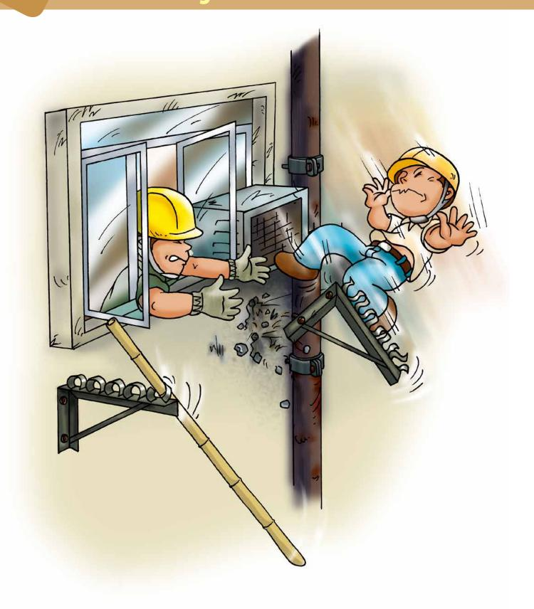
The drainage pipe on the external wall of an upper floor domestic unit was blocked. Two scaffolders, including the deceased person, were called in to erect a truss-out bamboo scaffold outside the unit to facilitate the clearing of the drainage pipe. The bamboo scaffold was erected in such a way that the two existing metal brackets of the laundry drying rack were used as part of the support for the scaffold.
