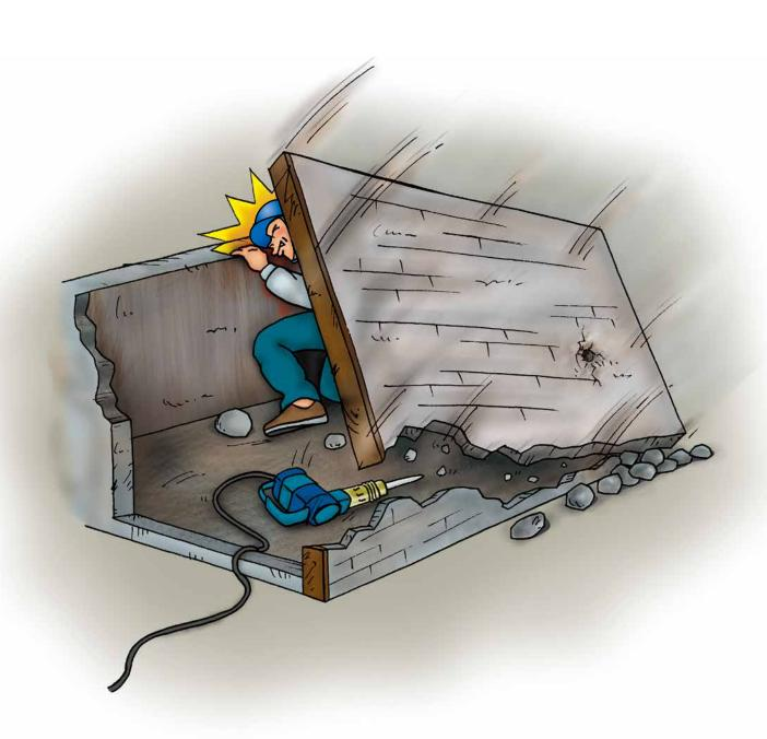
A contractor was appointed to demolish an unauthorized structure on the roof of a residential building. During the demolition, a worker was breaking a brick wall with a portable electric concrete breaker. The wall suddenly collapsed and struck the worker. Unfortunately, he was fatally trapped between the collapsed brick wall and a parapet nearby.
