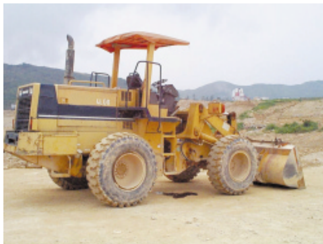
Fig.3 Check for leakage of lubricating or hydraulic oil, or coolant
