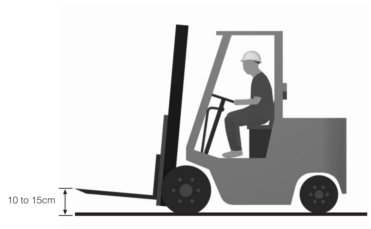
Figure 12 - Showing the position of the forks during travelling
