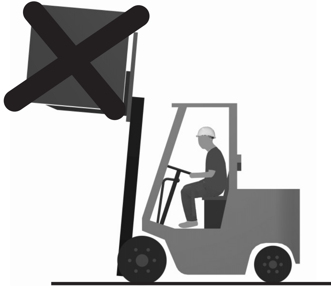
Figure 13 - Travelling with the load raised is dangerous
