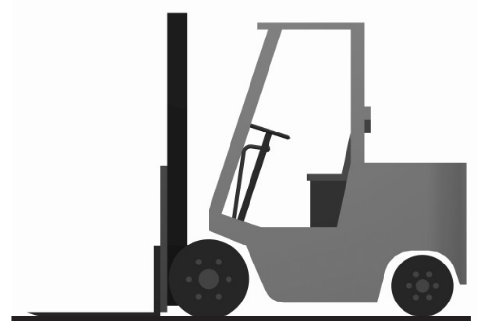
Figure 14 - The fork arms should be lowered to the ground/floor when unattended
