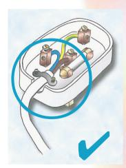
**4.** Secure the cores firmly to the respective plug pins / terminals in accordance with the following schedule:
