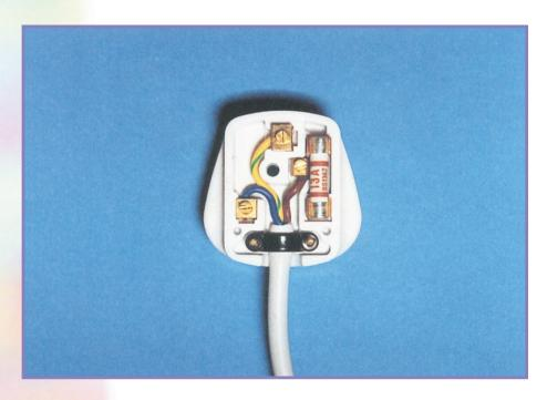
Warnings: Do not reverse the line (L) and the neutral (N) cores. Do not leave the earth core unconnected.
