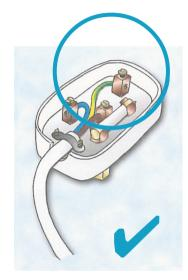
The insulation cover of the cord/cores should be removed with care to avoid cutting the strands of copper wires, or other damages.
