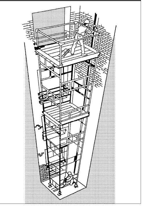
Note :For simplicity, illustrations on using additional guys, anchors, outriggers or kentledge for scaffold stability purposes have been left out in this figure.
