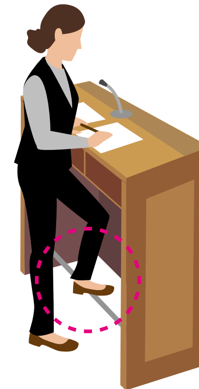
A foot-rail/footrest installed at a reception counter for the receptionists to rest their legs alternately.
