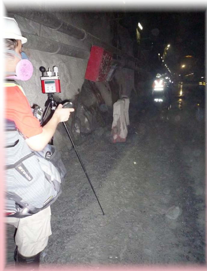
An occupational hygienist measuring air contaminants and the heat stress level in a tunneling work site
