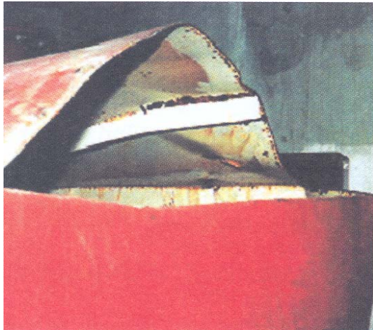
Photo 24.3 and 24.4 The blow-down tank was deformed and opened up
