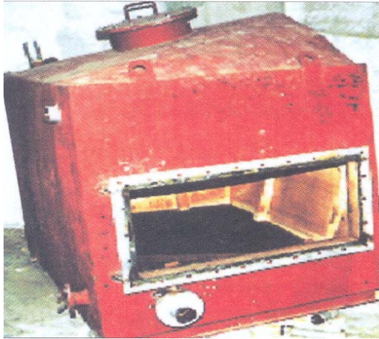
Photo 24.1 The blow-down tank was deformed and opened up
