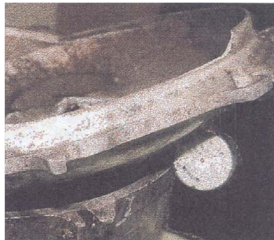
Photo 1.4 Broken lip seal rim of the lid
