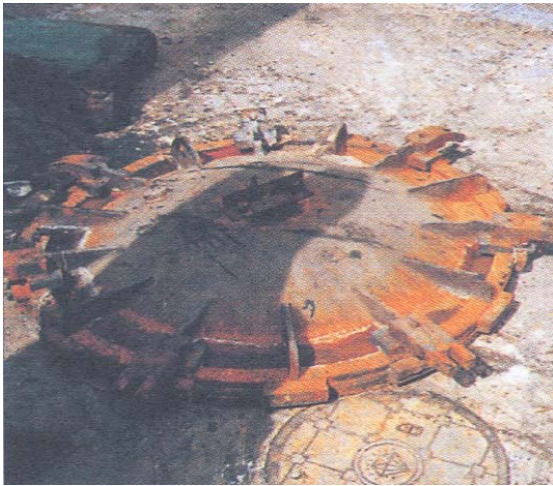
Photo 11.3 The bent cover lugs of the kler cover
