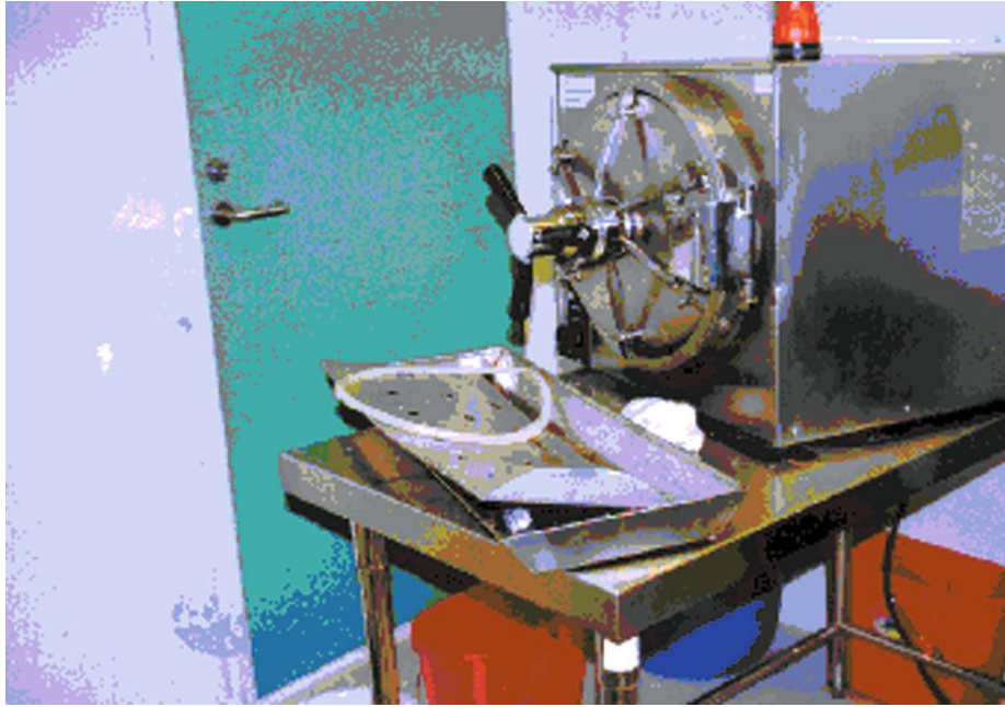
Photo 25.1 Autoclave door without pressure safety interlocking device
