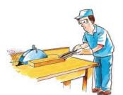
• The blade catches the timber and violently throws it back to the front of the saw, towards the operator.
